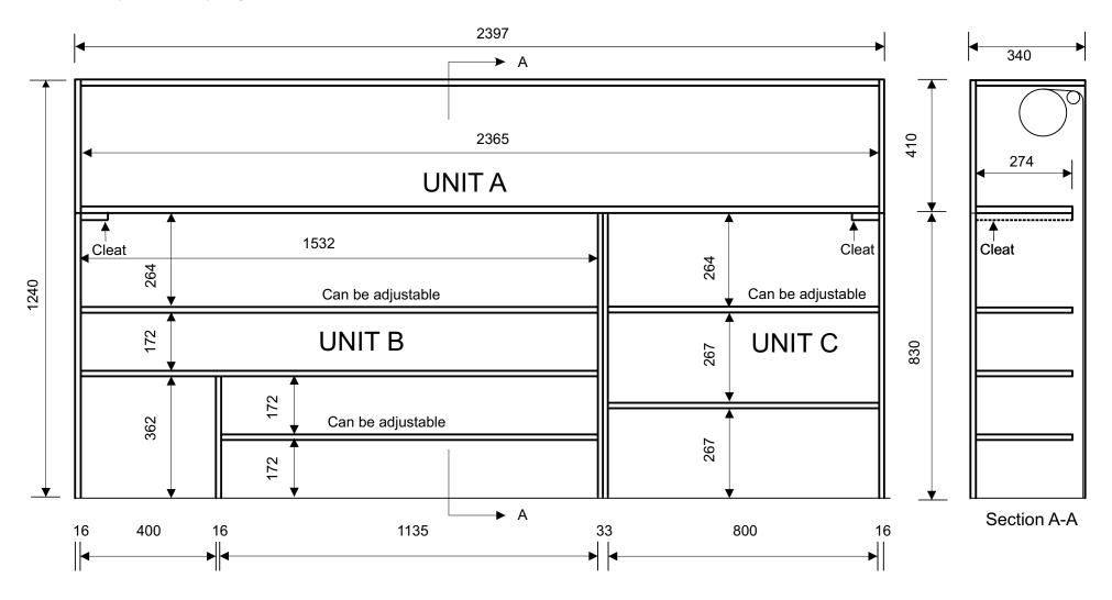
This drawing depicts the actual measurements of the smaller Benchtop Pantry shown in the Installation of an Electric Motor video.
