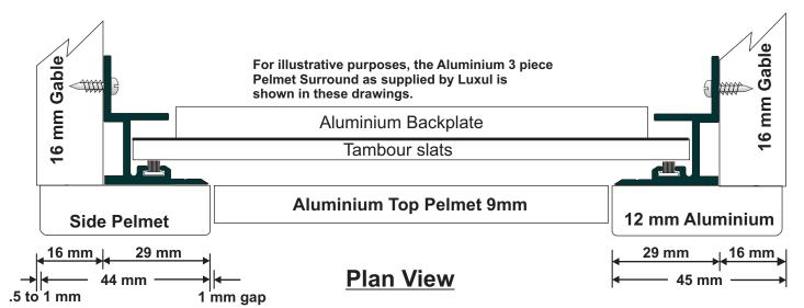
NOTE:- If you wish to screw-fix the Top of the Pelmet supplied By Others, the Pelmet HAS to be fitted & fixed BEFORE the FRONT ROLLER is fitted.
