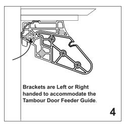
4 Fit the 2 part brackets flush to the carcass top and flush to the Blade/Gable front edge using adjustable screw slot [arrowed] first. Ensure the bottom section of the bracket is FIRMLY nested to the top section
