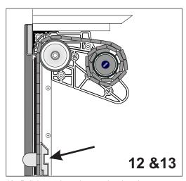
12 Pull the tambour down to the closed position and inspect the tambour door. Are there any gaps or lines in the face of the tambour. If so, there is rubbish between the slats. Un-install the Tambour door, remove the rubbish then re-install.
