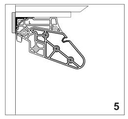
5 Slide the specially designed aluminium angle into position on top of the brackets DO NOT FIX.
