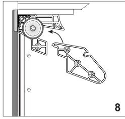
8 Remove lower section of one of the brackets and place front roller into roller slots. Refix lower section of bracket. Roller must spin freely.
