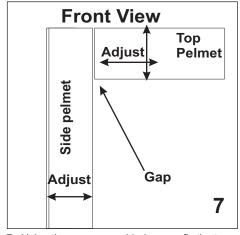
7 Using the screws provided, screw fix the top aluminium angle then, using the **BLACK** screws provided fit **your** own 1 or 3 piece Pelmet through the aluminium side tracks and the top aluminium extrusion.
