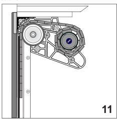
11 While maintaining the tension of the tambour door spring, CAREFULLY unroll the tambour door over the front roller and feed into the aluminium side tracks. The feeder guides on the brackets will point the 1st slat into the track.
