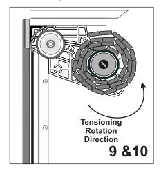
9 Unwrap the Tambour Door, ensuring no dust or particles fall in between the slats, and, from behind the brackets, place the door into the bracket slots. Apply pressure to the pin end to click into bracket
