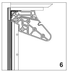
6 Slip the aluminium side tracks onto the locating tab of the brackets. Ensure track is FLUSH with front edge of Blade/Gable then screw fix. NOTE:- If Luxul 3 piece Pelmet Surround has been ordered, the Side Pelmets will be pre-fitted to the side tracks.
